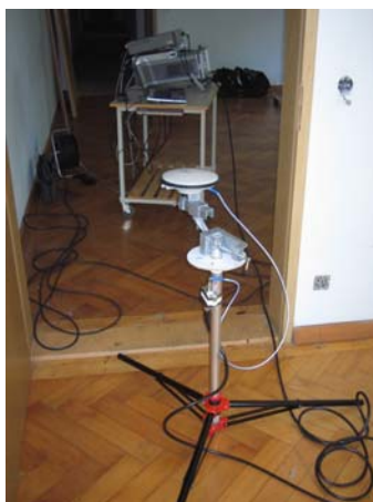
Equipment for the collection of Galileo signal spectra (Galileo antenna and spectrum analyser)
