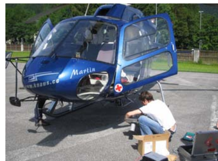
Installation of the Galileo transmit antenna at the left skid of the helicopter
